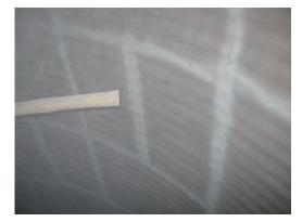
System: Surface preparation: Full blast to SA 2.5 and Rz 50-70μm ZINGA 1 x 60 μm DFT
