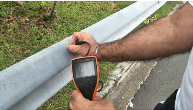
Condition survey of KAMPONG JAVA Road Rails in December 2017, 13 years after ZINGA application.
