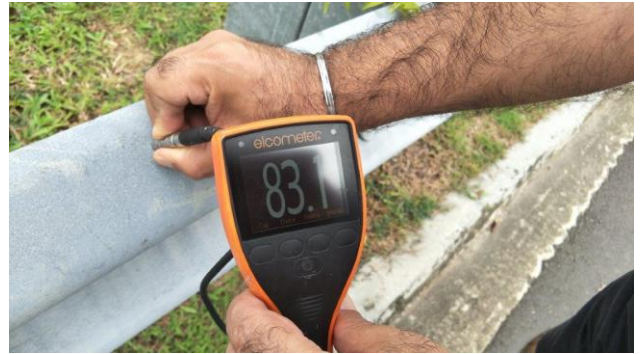
Condition survey of KAMPONG JAVA Road Rails in December 2017, 13 years after ZINGA application.
