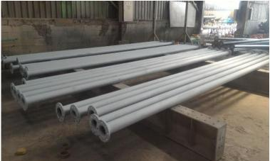
System:Blasting to SA 2.5 and Rz 50-70 μmZINGA1 x 100 μm DFTZINGACERAM HS1 x 100 μm DFTZINGACERAM PU1 x 80 μm DFT
