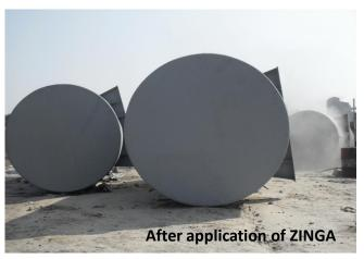
System: Surface preparation: Blasting to SA 2,5 and Rz 50-70µm ZINGA 2 x 60 µm DFT
