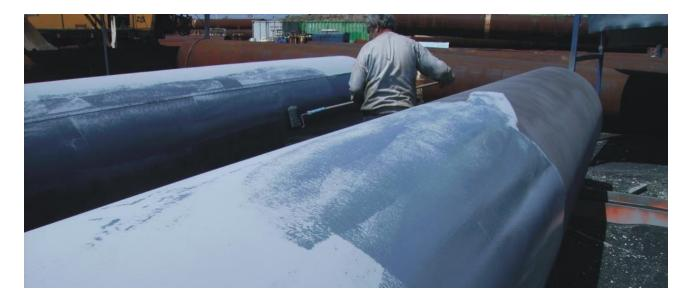
System: Surface preparation: SA 2,5 and Rz 50-70μm ZINGA 2 x 75 μm DFT
