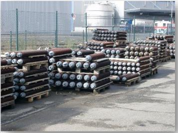
System: Surface preparation: SA 2,5 and Rz 50-70μm ZINGA 2 x 60 μm DFT
