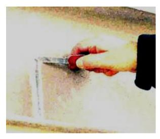
On this picture the dust is being removed and the intact **ZINGA** layer becomes visible.
