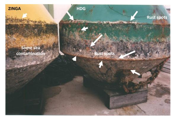
Conclusion of this test by the **DDE**: the buoy protected with **ZINGA** showed no trace of rust, but the hot-dip galvanised buoy was severely corroded in several places.
