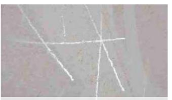
Photo Shows **ZINGA** "Film Galvanising". Scratched with a coin to show the pure active zinc exposed.
