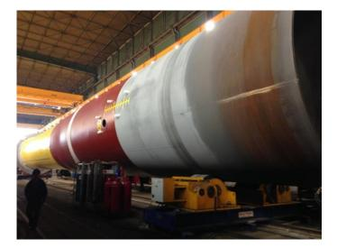
In 2014 **ZINGA** was used on the construction of new windmills for Dutch energy provider **ENECO**. **ZINGA** was chosen to protect the most sensitive parts of the windmills: the monopile's external primary steel, +3m up the mudline to -2m below the mudline. The top of the monopile flange was protected with **ZINGA** (2 x 90 µm DFT).
