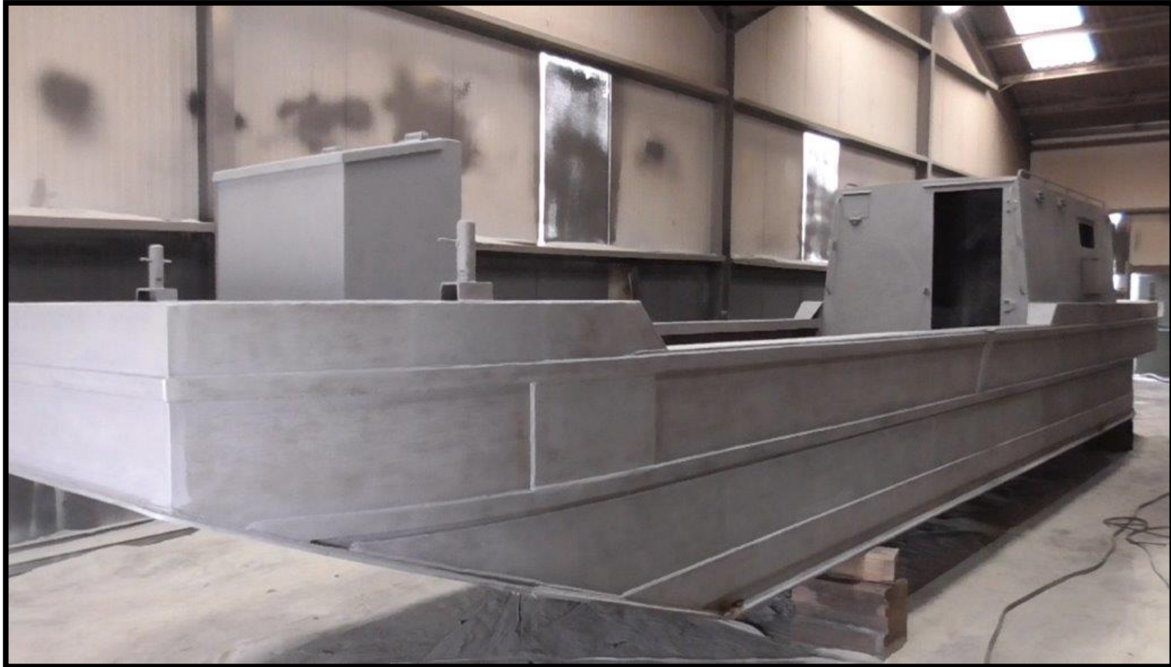
The first of 200 canal work-boats to use the Zinga system
