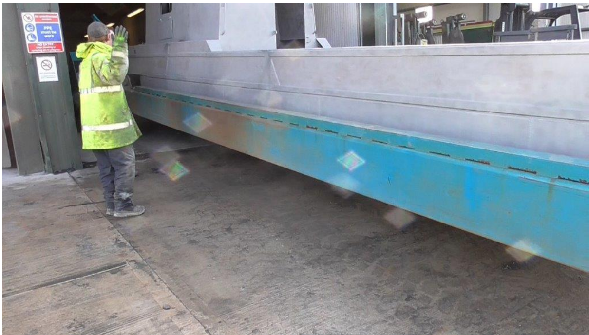
Transferring the work-boat from the blast-shop to the paint-shop. Tarpaulins are used in wet weather
