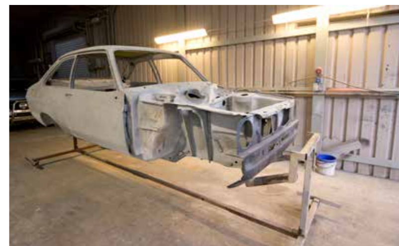
This RS2000 has been sitting in bare steel for over a year. The Zinga application has kept it completely rust-free since then.
