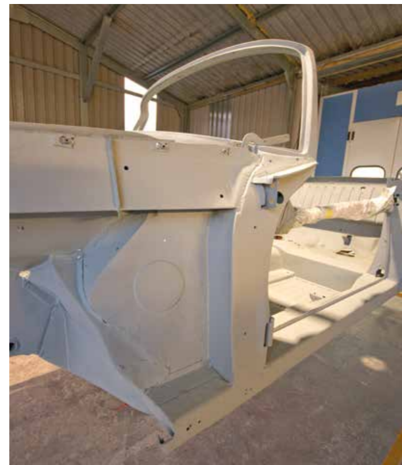
Kieran and his team normally spray the Zinga onto the bare metal due to the size of the projects they're working on, but it can be brushed on just as well. As you can see here, no corrosion has crept back on the bare steel.
